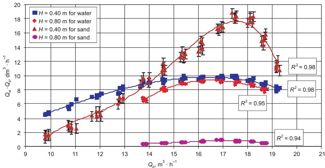
**Fig. 5.** Water flow rate  $Q_w$  and sand flow rate  $Q_s$  vs. air flow rate  $Q_p$
